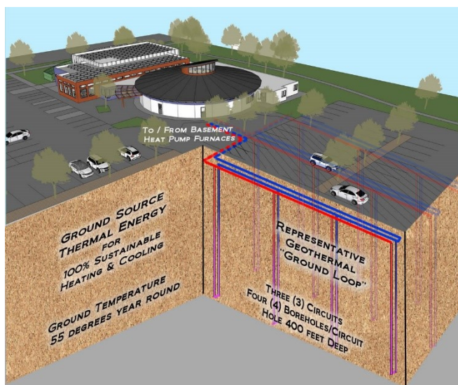
Figure 36 Energy System Concept (Solar & Geothermal)
